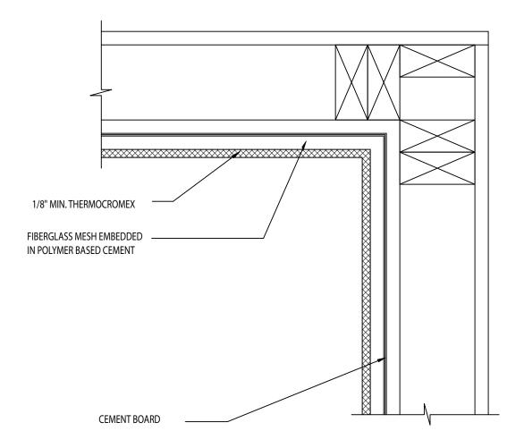
NOTE: All joints of cement board must be treated with 4" fiberglass mesh embedded in polymer based cement.
